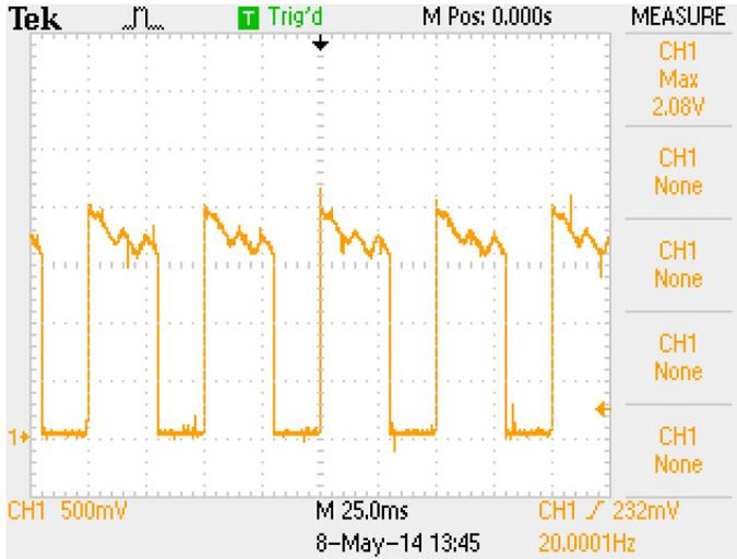
Figure 2: Voltage at IO representing the output current waveform: 280V / 60% / 20Hz
