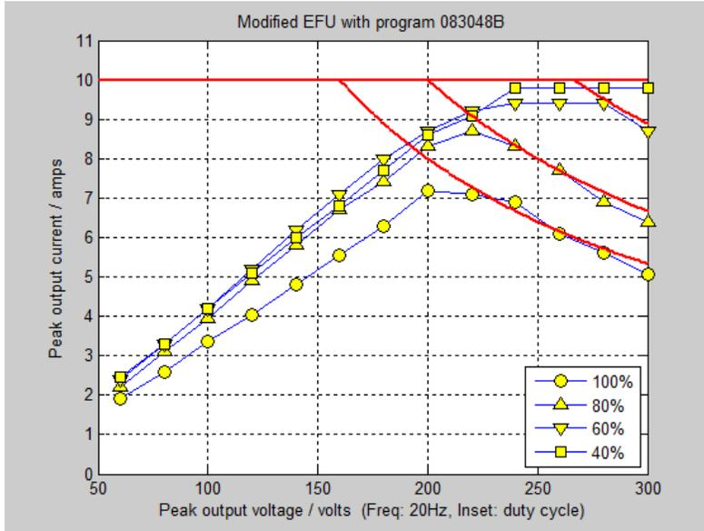
Figure 12: Peak output current vs peak output voltage at 20Hz for various of duty cycles. The three solid red lines at the top right hand of the graph represent the maximum current limit for a power dissipation of 1600W for the duty cycles 100%, 80% and 60%.
