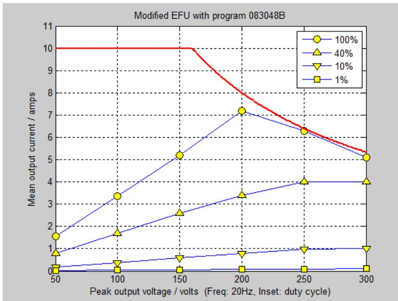
Figure 11: Mean output current vs peak output voltage at 20Hz for various duty cycles
