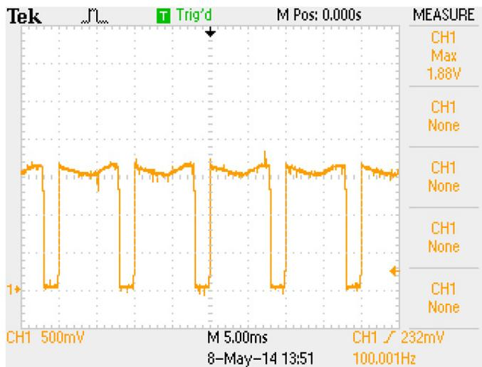
Figure 7: Voltage at IO representing the output current waveform: 260V / 80% / 100Hz (Note the faster modulation frequency)
