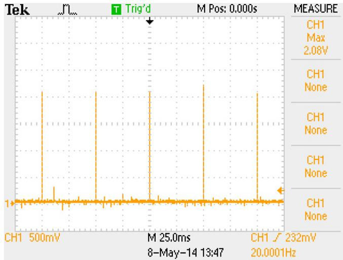
Figure 5: Voltage at IO representing the output current waveform: 260V / 1% / 20Hz
