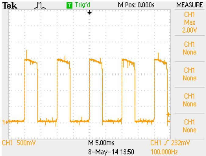
Figure 8: Voltage at IO representing the output current waveform: 260V / 40% / 100Hz (Note the faster modulation frequency)
