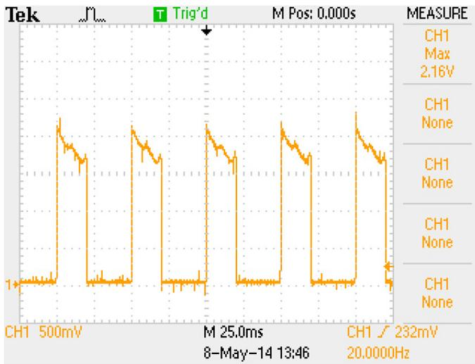
Figure 3: Voltage at IO representing the output current waveform: 300V / 40% / 20Hz
