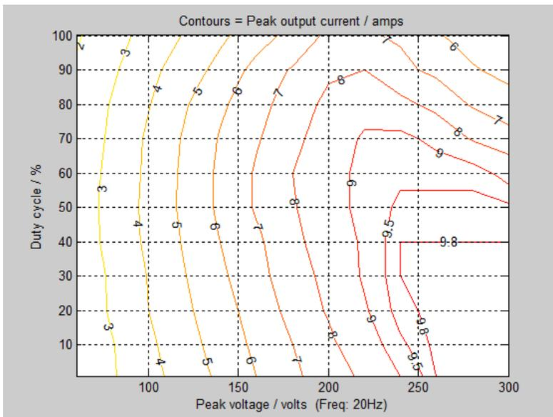
Figure 13: Peak output current contours for various peak output voltages and duty cycles. The modulation frequency is 20Hz.
