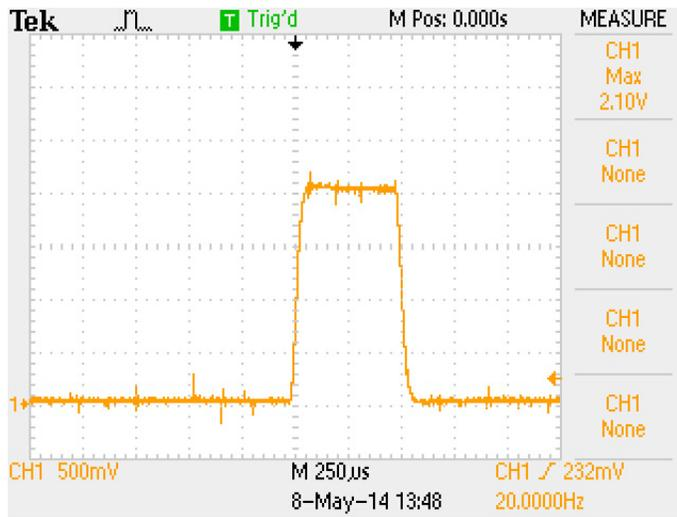
Figure 6: Voltage at IO representing the output current waveform: 260V / 1% / 20Hz (as above but with faster timebase)
