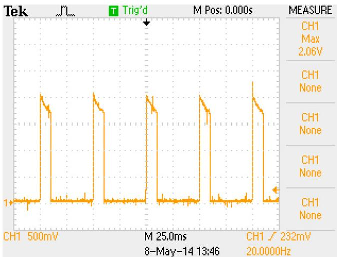
Figure 4: Voltage at IO representing the output current waveform: 240V / 20% / 20Hz
