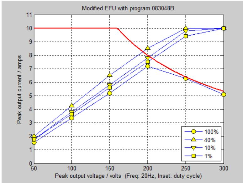
Figure 10: Peak output current vs peak output voltage at 20Hz for various duty cycles
